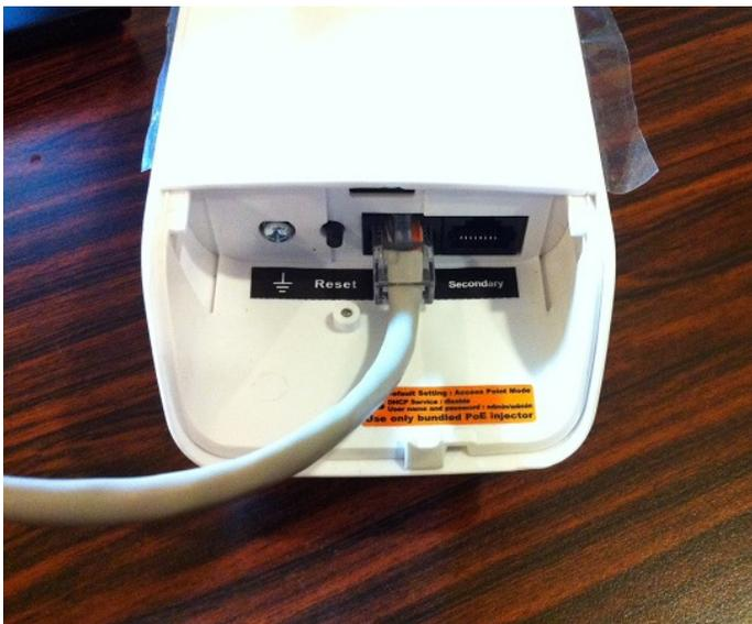
Note. LP-2396K built in PoE pass through function on Secondary Ethernet port. It means the Secondary Ethernet port is able to provide 24V power for a secondary device if this function enabled on Web Configuration (Please refer to the statement on Advanced Setting of Radio menu).
