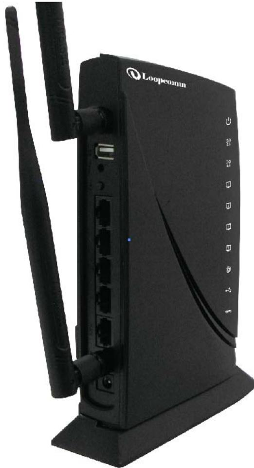
**Antenna Connectors (1-2):** RJ-SMA antenna connectors. Attach the included high gain dual band antennas to these connectors
