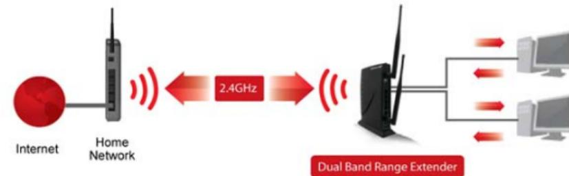
If you have configured the Dual Band Range Extender / Repeater to connect to a single band Home Network or if a connection is dropped from a dual band Home Network connection, the Dual Band Range Extender / Repeater will automatically default this setting to the Home Network connection that is active. For example, if the Dual Band Range Extender / Repeater is connected to a 2.4GHz Home Network only, it will automatically route all wired connects through the 2.4GHz Home Network connection.
