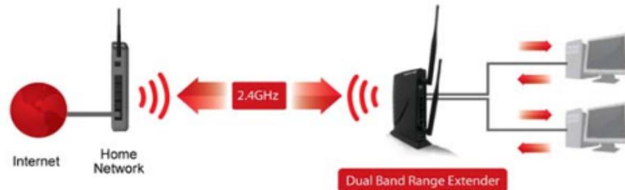
If you have configured the Dual Band Range Extender / Repeater to connect to a single band Home Network or if a connection is dropped from a dual band Home Network connection, the Dual Band Range Extender / Repeater will automatically default this setting to the Home Network connection that is active. For example, if the Dual Band Range Extender / Repeater is connected to a 2.4GHz Home Network only, it will automatically route all wired connects through the 2.4GHz Home Network connection.
