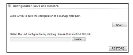
Save: Press Save button to save the current configuration settings of the device to the Management Host or click the *Browse* button to locate the configuration file,
