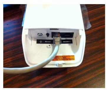
Note. LP-2396K built in PoE pass through function on Secondary Ethernet port. It means the Secondary Ethernet port is able to provide 24V power for a secondary device if this function enabled on Web Configuration (Please refer to the statement on Advanced Setting of Radio menu).
