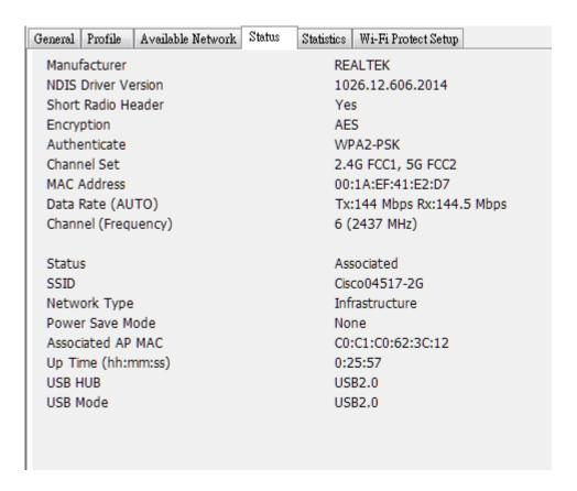
In this page, it shows all wireless, networking and device driver version of 802.11n 5GHz in detail
