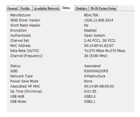
In this page, it shows all wireless, networking and device driver version of 802.11ac 5GHz in detail.
